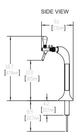
For connection to Elkay **CARBONATION CHILLER** only. Not to be connected directly to main water supply or other chillers Customer to provide mounting hole in countertop. Mounting hole diameter 1-3/8" to 1-1/2". Additional support is recommended for sheet metal or counter tops under 3/4" thick
