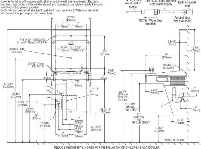
A = Recommended Water Supply location. Shut-off Valve (not furnished) to accept 3/8" O.D. unplated copper tube. Up to 3" (76mm) maximum out from wall.
