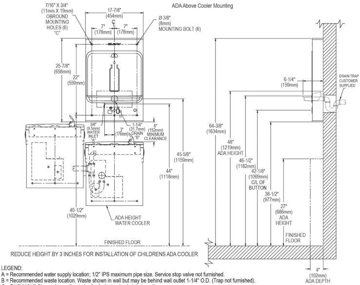
C = 7/16" X 3/4" Obround mounting holes for fastening backplate to wall.
