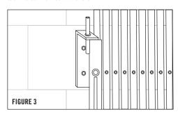
**4)** Extend and retract gate to its stops to work out stiffness, then fully extend gate across opening. Align padlock holes and position the locking bar on door frame or wall. Mark and drill pilot holes. Secure with 5/16" x 2" lag bolts. (See Figure 4)
