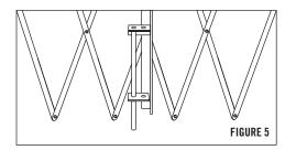
6) Gate can be secured to locking bar using padlock. Open gates slowly at first to avoid warping.
