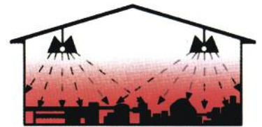
INFRARED HEAT Infrared heat works from the bottom up, warming people, floors, objects and machines first. Comfortable heat is retained in the lower working areas of your building.
