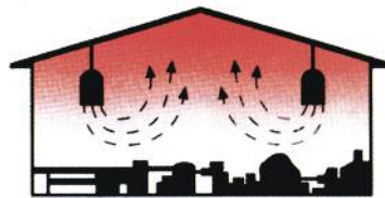
CONVECTION HEAT Forced air convection heat works from the top down, heating the air first and stratifying from the ceiling downward. More heat is wasted in the upper area the building.
