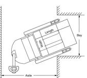
Aisle dimensions listed above assume the minimum bay width to be straddle OD plus 5" (2.5" on each either side of straddle leg). Straddle OD is the load width plus 8". Truck performance may vary due to application requirements' and changes in model design.
