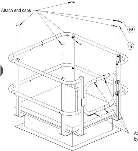
Adjust swing gate to the proper opening by loosening the (4) screws and make adjustment
