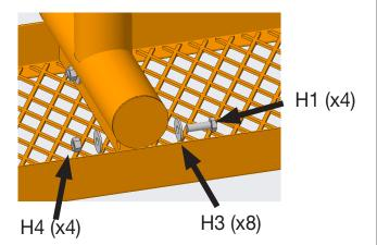
2. Attach leg supports to both legs and bench top (3 points) with the hardware provided. Use images below as reference.
