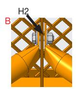
3. Insert 2 steel bars (Ref.5) through the bottom of each leg. Steel bars must be symmetrically placed in order to function adequately during in-ground installation. Steel bar must remain symmetric while in leg.
