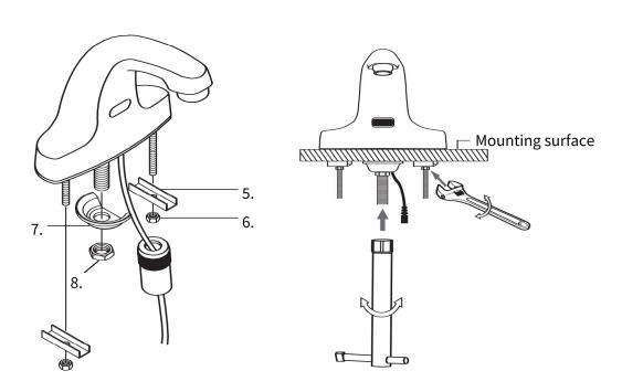
Thread sensor cable and shank through the mounting hole, make sure spout body & base gasket are flat on the mounting surface. Secure using fixation nuts & gaskets per this diagram.
