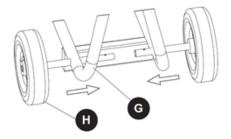
2. Secure wheels (H) by inserting a split pin (AA) into the whole on the wheel shaft and splitting the pin.
