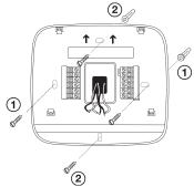
top and one screw on the bottom. For horizontal mount put one screw on the left and one screw on the right.
