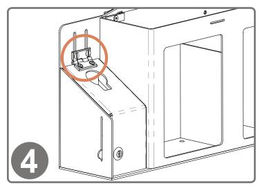
Once mounted, load consumables. Bottle cover height is adjustable by loosening top screws on hinge and sliding along slots. Tighten when desired height is set.
