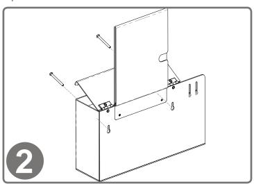
Dispenser can also be mounted securely to a wall through keyholes and screw holes in back with screws approved and supplied by building maintenance.
