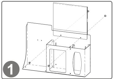
To mount the MP-075 Sign Holder, align the holes of the holder with the holes of the dispenser. With a flathead screwdriver, attach using (2x) barrel screws included with sign holder.
