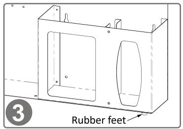
For placing on counter, attach (4x) self-adhesive rubber feet at each of the bottom corners (included).
