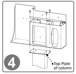
Attach the RS005-0223 Respiratory Hygiene Station to the column using (4x) screws included with stand. Tighten.
