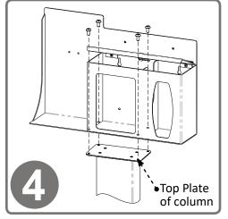
Attach the RS005-0212 Respiratory Hygiene Station to the column using (4x) screws included with stand. Tighten.
