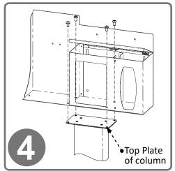
Attach the RS005-0412 Respiratory Hygiene Station to the column using (4x) screws included with stand. One pair of screw holes is located in the hand sanitizer dispener section; the second pair are inside the facemask section and can be accessed with the lid open. Tighten all screws.
