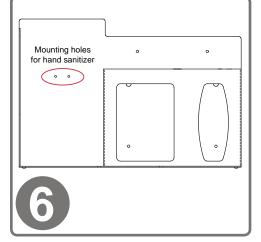
Attach hand sanitizer dispenser using VHB tape or mounting holes provided.
