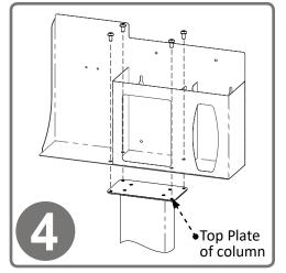
Attach the RS004-0212 Respiratory Hygiene Station to the column using (4x)screws included with stand. Tighten.
