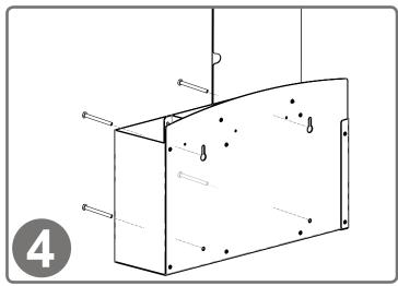
Dispenser can also be mounted securely to a wall through keyholes and screw holes in back with screws approved and supplied by building maintenance. All four mounting holes provided must be used.
