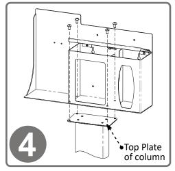
Attach the RS005-0233 Respiratory Hygiene Station to the column using (4x) screws included with stand. Tighten.
