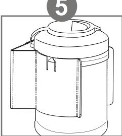
Slide wipe canister into dispenser from top down until pointed notch locks into rib or lip near the lid of the canister.
