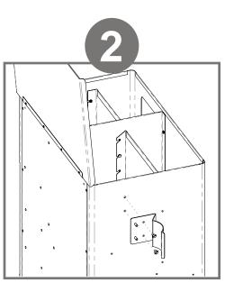
Attach bracket to cart through prethreaded holes on left side of cart as shown.
