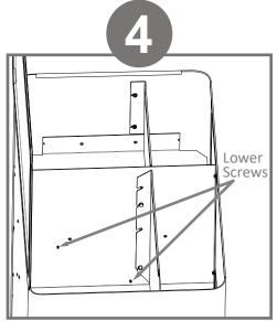
Keeping the rounded corner at the top left, reposition divider at a slanted position, resting on lower screws.
