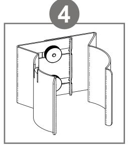
Determine size needed for disposable wipe canister and tighten plastic knobs at position needed to accommodate canister.
