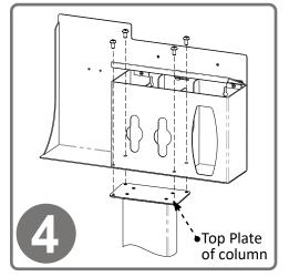
Attach the RS013-0212 Respiratory Hygiene Station to the column using (4x) screws included with stand. Tighten.
