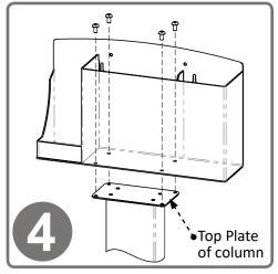
Attach the RS001-0512 Respiratory Hygiene Station to the column using (4x) screws included with stand. Tighten.
