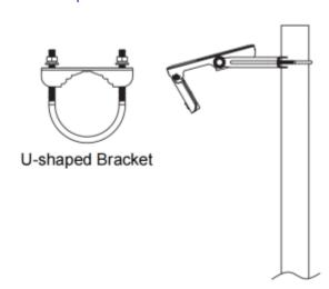
Please use 2pcs U-shaped bracket to mount the lamp onto the pole.
