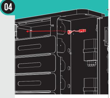
Take out the cable through the hole, replace with new cable and plug back into USB port. Make sure to close cable grip when finished.
