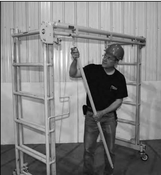
6) Attach braces between the beam and the base of each end section. WARNING: NEVER operate the Tele-Tower Adjustable Work Platform without these braces. Doing so can result in damage to the structure which can lead to failure that can result in severe property damage and/or severe bodily injury or death.
