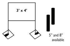
3', 4', 6'6" bases are designed to overlap so the barriers are seamless when aligned with one another.
