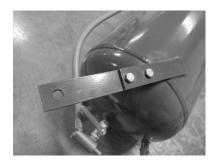
2. Connect axle support bracket (Ref 2) to tank (Ref 23) using hex bolt (Ref 6).
