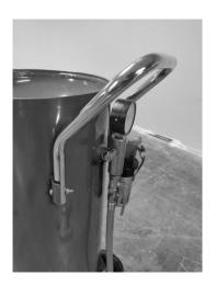
6. Attach tank handle (Ref 14) to tank using M6 bolt (Ref 18), washer (Ref 17), and nut (Ref 19).
