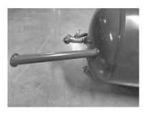
1. Connect tank foot (Ref 24) to tank (Ref 23) using cotter pin (Ref 5).
