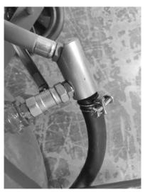
5. Attach hose clamp (Ref 27) and abrasive hose (Ref 25) to tee joint manifold (Ref 26) .
