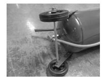
4. Insert axle (Ref 1) through the support brackets and assemble the other wheel assembly..
