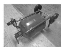
3. Place tank (Ref 6) on the floor and lay axle bracket assembly on the fastening points. Fasten the bracket to tank with the M6 screw (Ref 8), washer (Ref 7), and nut (Ref 9).
