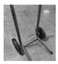
1. Insert axle bracket (Ref 5) into both ends of the wheel axle (Ref 4). Ensure that fastening holes on axle bracket point outwards.
