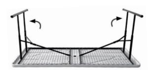
Ensure that the diagonal braces are in locked position.
