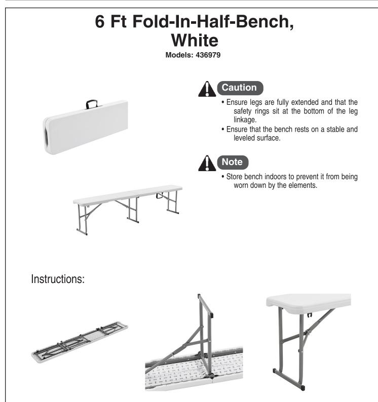
2. Open each leg, fully extending the leg and linkages.
