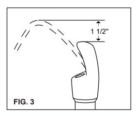
**CAUTION:** The fountain is rated for inlet water pressure of 20-105 PSI. A pressure reducing regulator should be used if the inlet water supply exceeds 105 PSI. Any damage caused by reason of connecting this product to supply line pressures lower than 20 PSI or higher than 105 PSI will void warranty.
