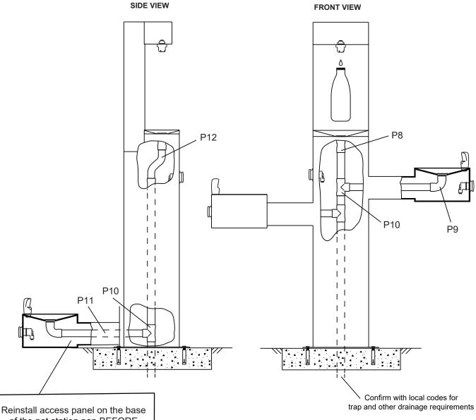
Reinstall access panel on the base of the pet station pan BEFORE connecting (P11) Drain Tube to (P10) T-Shape Drain Connector; using (8) M6 x 10 flat-head antitheft screws preciously removed.
