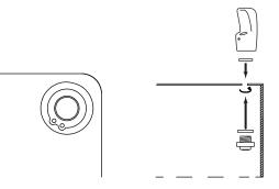
**2b.** Locate the hole on the drinking fountain pan surfaces. Align and sanwich with the two washers and tighten the nut to secure the bubbler.
