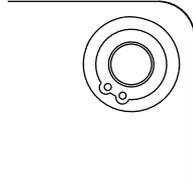
**2b.** Locate the hole on the drinking fountain pan surface. Align and sandwich with the two washers and tighten the nut to secure the bubbler.
