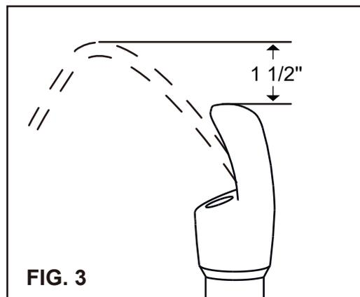
**CAUTION:** The fountain is rated for inlet water pressure of 20-105 PSI. A pressure reducing regulator should be used if the inlet water supply exceeds 105 PSI. Any damage caused by reason of connecting this product to supply line pressures lower than 20 PSI or higher than 105 PSI will void warranty.
