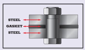
**SOFT PULL-UP** – More deflection occurs during torqueing at greater than 720 degrees after contact.
