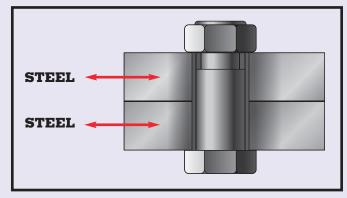
**HARD PULL-UP** – Minimal deflection occurs during torqueing at less than 90 degrees after contact.
