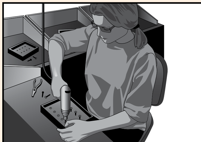
Application: Securing an electronic board to blind holes in a plastic frame
