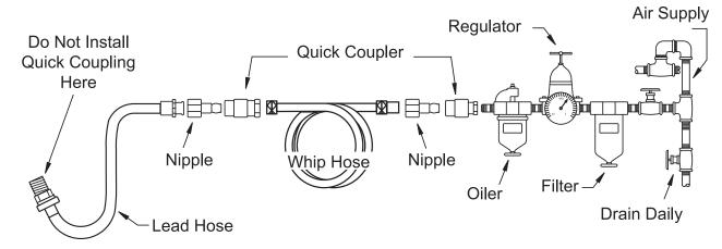
The air inlet, used for connecting the air supply, has standard 1/4" NPT American Thread.
