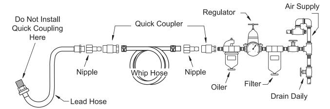
The air inlet, used for connecting the air supply, has standard 1/4" NPT American Thread.
