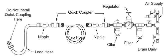
The air inlet, used for connecting the air supply, has standard 1/2" NPT American Thread.
