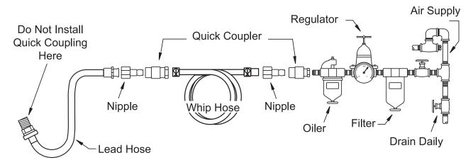
The air inlet, used for connecting the air supply, has standard 1/2" NPT American Thread.
