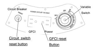
A ground-fault circuit interrupter detects an abnormal current flow to ground and opens the circuit, preventing a hazardous situation.
