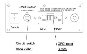
A ground-fault circuit interrupter detects an abnormal current flow to ground and opens the circuit, preventing a hazardous situation.
