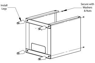
**Step 3** Move into position and level front to back, side to side.
