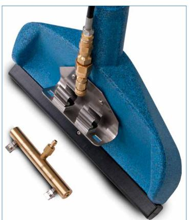
Talk about durability, the wand shoe is made of UHMW plastic which has the highest impact strength of any thermoplastic presently made. The wand glides easily across the carpet and wears less because the UHMW plastic shoe also has an extremely low coefficient of friction. For example, it is significantly lower than Delrin and other Acetals.
